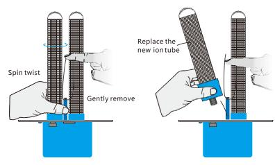
1.Gently move away the power sheet metal, Pinch the ion tube counterclockwise twist for a few turns, you can take it out.
