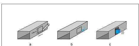
1.If the space is not enough, the equipment can't be installed in the pipe, please see the other install method below
